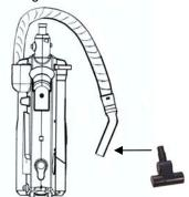
Important: In order to ensure that maximum air suction is maintained. empty the dust cup frequently and shake out the HEPA filter and clean the nonwoven pre-filter and debris screen at the same time. Ensure that the rotating brush is kept free of hair and string which may accumulate and decrease brush performance.
